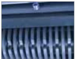
Specially developed cutting and perforating rollers
